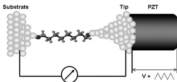
**Figure 1.** Schematic illustration of a single-molecule conductance measurement with contact configuration modulations. The experiment was carried out by superimposing a small ac voltage to the piezoelectric transducer (PZT) while repeatedly stretching the molecular junction using the STM break-junction method.
