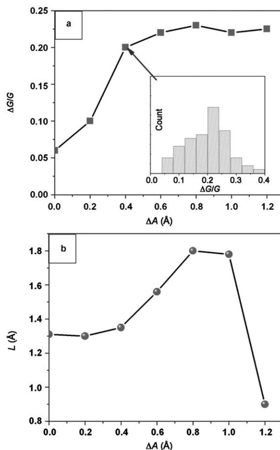
**Figure 4.** a) The relative single  $C_8$ -molecule conductance fluctuation amplitude ( $\Delta G/G$ ) versus PZT modulation amplitude ( $\Delta A$ ). The value of  $\Delta G/G$  used in the plot was determined using peak values in the  $\Delta G/G$  histograms (see inset). b) The stretching length ( $L$ ) of the single  $C_8$ -molecular junction versus PZT modulation amplitude.
