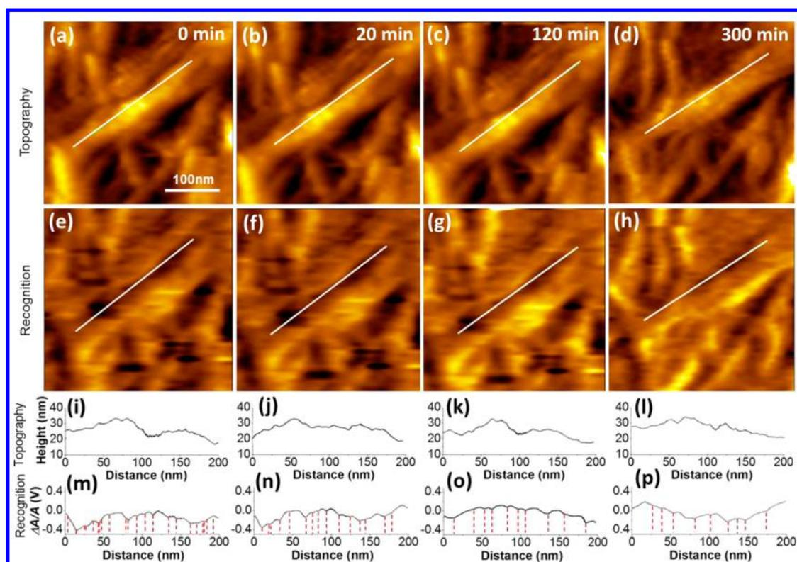
**Figure 2.** Timeline of CBM3a binding to crystalline cellulose: (a–d) topography images; (e–h) recognition images; (i–l) cross sections of topography images along the white lines; (m–p) cross sections of recognition images along the white lines. Some representative binding sites are labeled with red, dashed lines.
