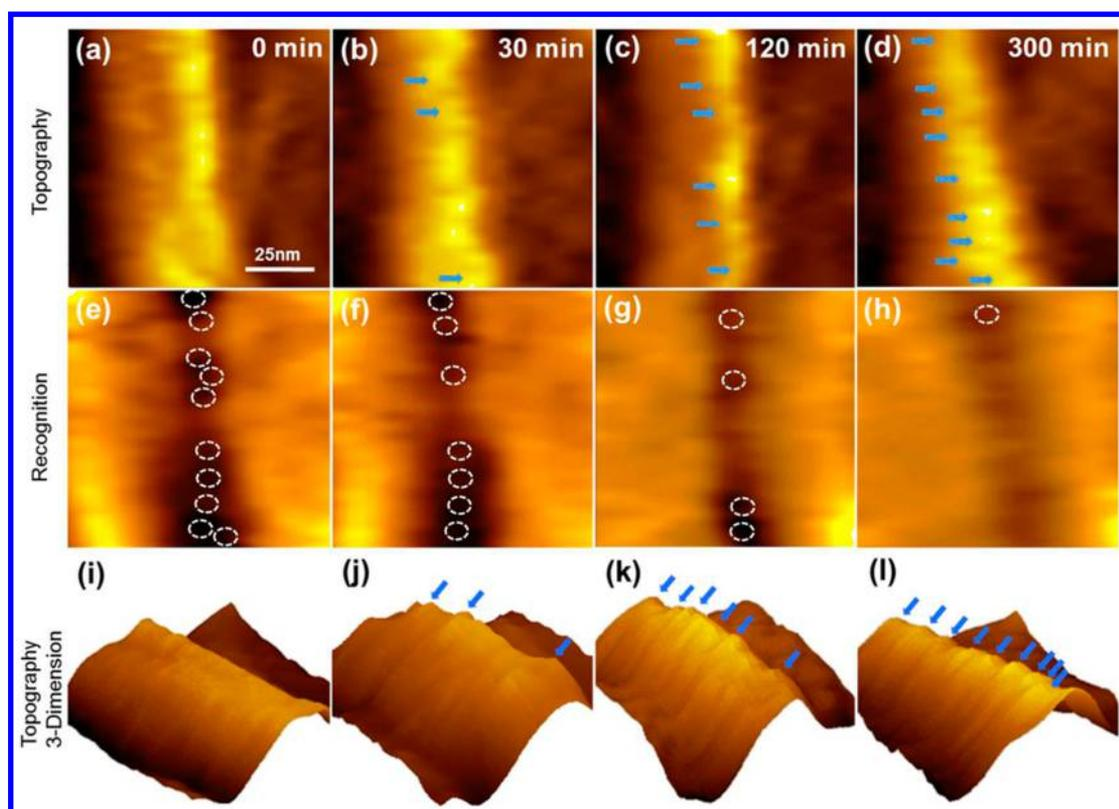
**Figure 3.** AFM topography (a–d), recognition (e–h), and 3D (i–l) images of CBM3a–cellulose binding at a smaller scale. The blue arrows in (b–d) and (j–l) indicate the regularly aligned CBM3a molecules binding on a crystalline cellulose fibril from 0 to 300 min. The binding sites are labeled by white, dashed circles.
