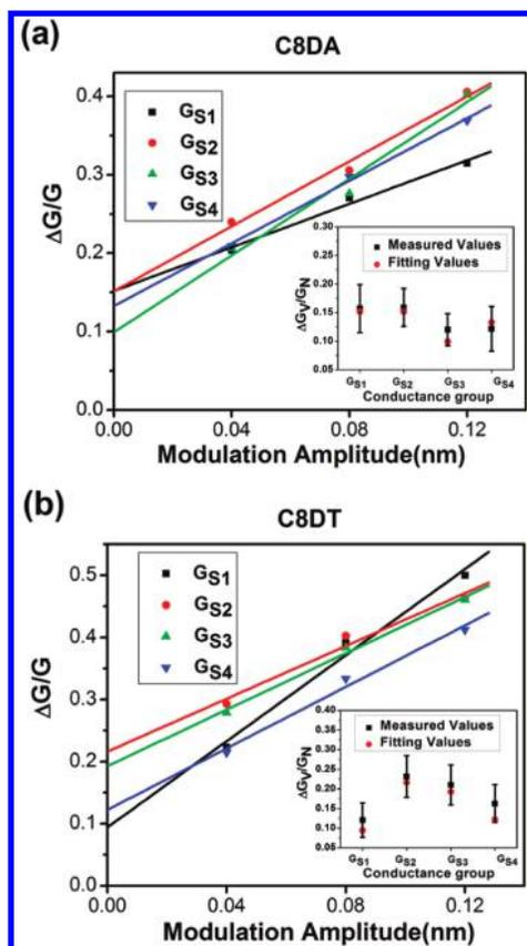
**Figure 4.** Linear fitting for relative conductance fluctuation amplitude versus modulation amplitude for C8DA (a) and C8DT (b). The different conductance sets are labeled with different colors. The insets compare the fitting  $\Delta G_V/G_L$  (red) values and the measured  $\Delta G_V/G_L$  (black) values.
