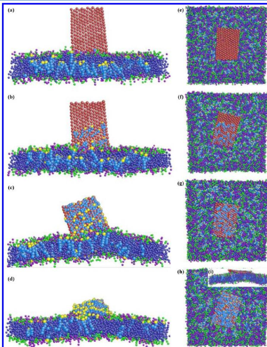
**Figure 4.** Orientation of graphene sheet (a)–(d) vertical orientation; (e)–(h) horizontal orientation; (i) cross-section view of horizontal orientation.
