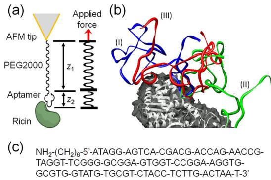
FIG. 1. The force-extension model for the aptamer-ricin interactions. (a) The series-spring model. (b) The simulated aptamer-ricin binding conformations, where the aptamer conformations are labeled as (I) for pathway 1, (II) for pathway 2, and (III) for pathway 3. (c) The sequence of the aptamer modified with amino functional group.
